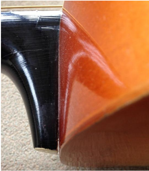
Photo 4: The neck heel had shrunk back from the body leaving a gap at the end of the heel.
