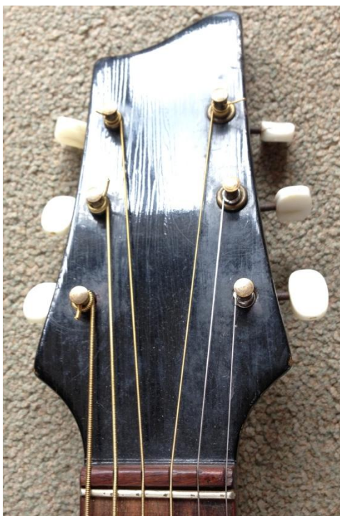
Photo 6: Only 2 of the tuners had their bushes. The others had no support & so the pull of the strings was deflecting the shafts & causing the holes in the head to be worn out of shape.
