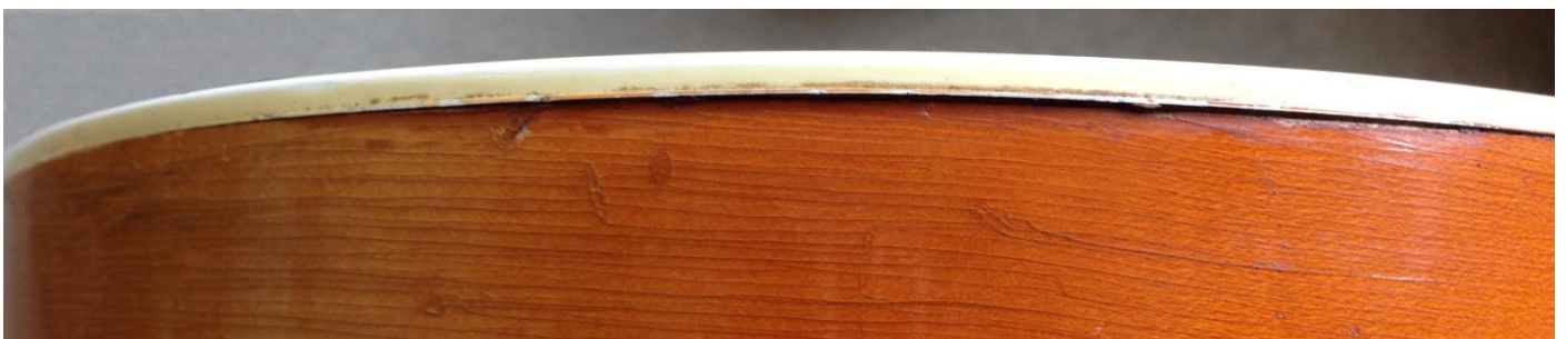
Photo 3: The front & binding had lifted around the lower bout.
