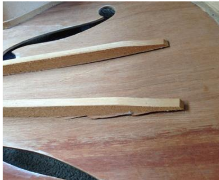
Photos 11 & 12: With the back off it was possible to assess the damage to the braces. One of them just had a failure of the glued joint but the other had partially ripped the surrounding surface. Both relatively easy to resolve.
