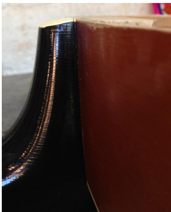
Photo 16: The neck heel required shimming to plug the gap caused by shrinkage. The neck joint itself was still tightly adhered & stable so didn't need any further attention. A tapered shim about 15mm long was pressed into the gap & glued in position.
