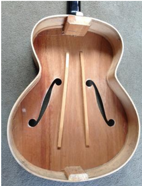
Photos 11 & 12: With the back off it was possible to assess the damage to the braces. One of them just had a failure of the glued joint but the other had partially ripped the surrounding surface. Both relatively easy to resolve.
